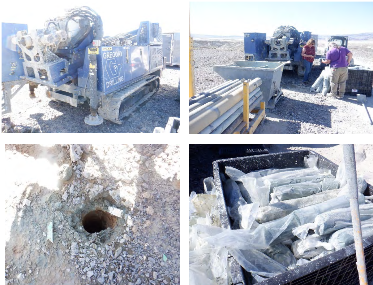
Figure 10-2: Sonic Drilling Rig and Equipment, Collar Hole, and Sonic Samples (Source: GRE, 2022)
